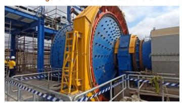
Image: Crushed rock feed to SAG mill
