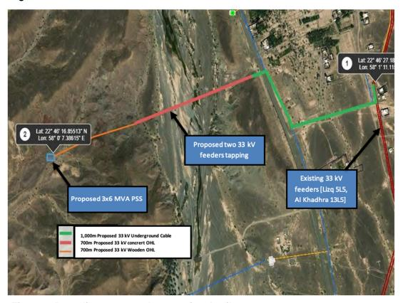
Figure 2: Powerline routes and connection details.
