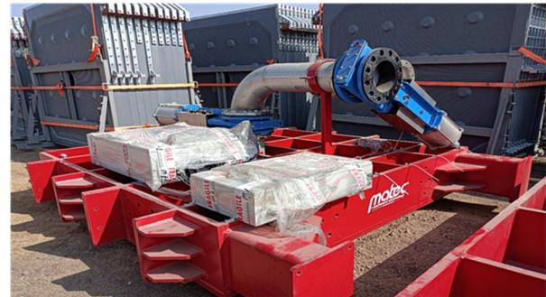
**Pressure filter 2500 – slurry feed distributor**
