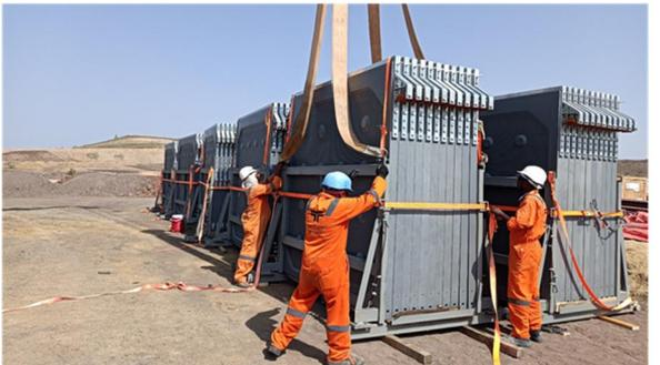
**Plates for pressure filter 2500 (Matec)**
