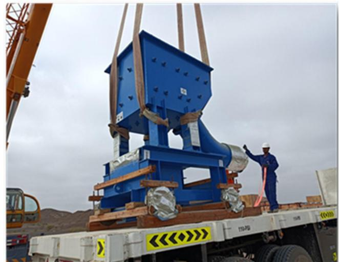
**Feed trolley assembly (ball mill)**
