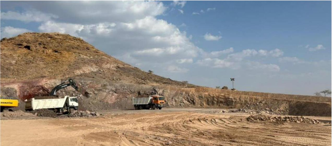
*First cut mining activities and overburden and limited oxide copper ore removal*
