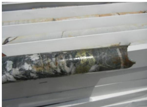
Drill Hole core from Zone 3 showing chalcopryite veins
