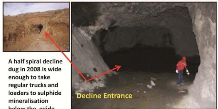
A half spiral decline dug in 2008 is wide enough to take regular trucks and loaders to sulphide mineralisation below the oxide cap, which covers most of the hill .
