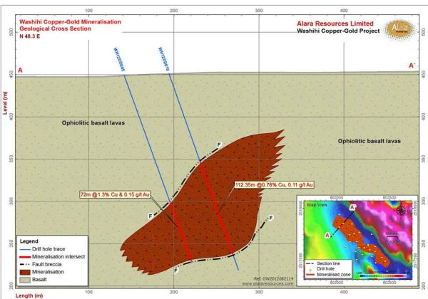
Figure 3: Cross section along 250N indicating a modest strip ratio
