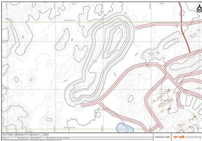
Figure 2: Mineralised Zone K2 Pit design plan
