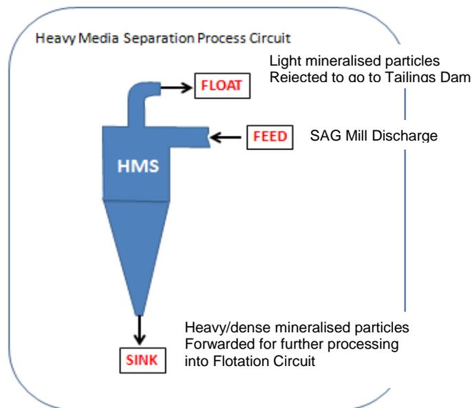
**Figure 3: HMS Process Circuit**
