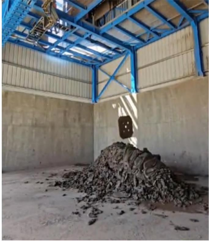
**Image: Processed Tailings Transported to Onsite Storage Facility**
