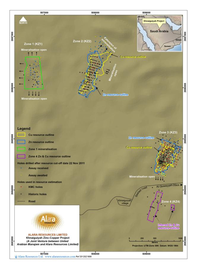
Figure 1 Location of Mineralised Zones 1 to 4 (KZ1 to KZ 4), Resource Outlines and Drill Hole Locations
