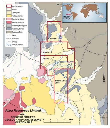
Lituania 3 concession, comprising 19 lines (with a grid of 50 x 20 metres) covering line 20 kilometres with 946 points of radiometric measurements taken (including a radiometric sweep between lines.
