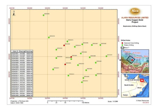
Figure 15: Daris East Prospect - 24 Hole Initial Drilling Programme
