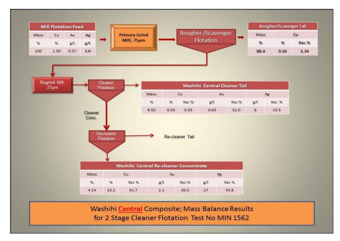
Figure 1 - Process flow sheet and mass balance for Washihi
