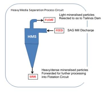
Figure 3: HMS Process Circuit
