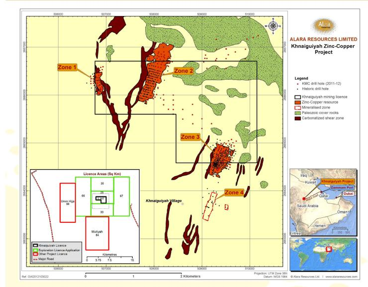
Zinc and copper mineralisation is focused along the carbonatised shear zones.
