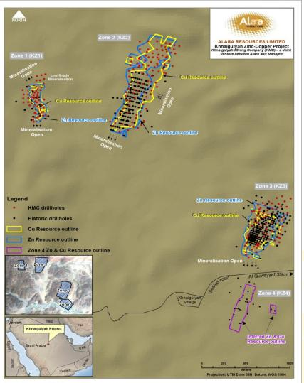
Total drilling: 71,816m in 622 drill holes
