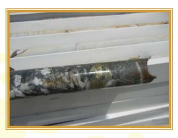
Drill Hole core from Zone 3 showing chalcopyrite veins
