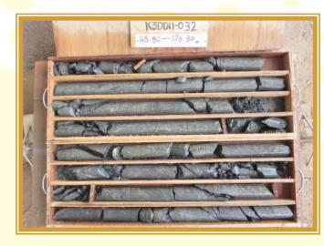
High grade zinc and copper intersections in Drill Hole K3DD11\_032 at Zone 3
