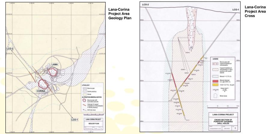
Two drill holes intersected 180m and 130m of mineralisation respectively, at 0.70% Copper and up to 200ppm Molybdenum
