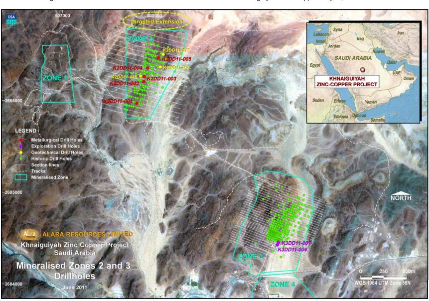
Figure 1 – Drill Hole Locations at Mineralised Zones 2 and 3 at Khnaiguiyah Zinc-Copper Project, Saudi Arabia
