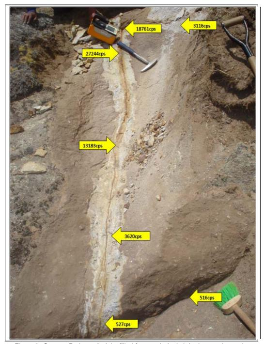
Figure 2. Crucero Project - Autinite-filled fracture in Ignimbrite host rock, as shown by anomalous spectrometer readings (measured in total counts per second (cps)).
